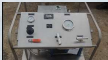
Chemical Injection Pump
